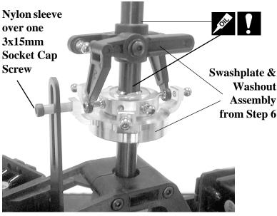
Completed Rotor Head Assembly from
