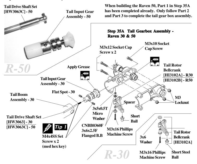
**Part1.** Raven 30, attach the tail input gear assembly on to the drive shaft with two 4x4mm Set Screws (**Tip 1**) (make sure the flat spot is aligned with one of the set screws and only use ONLY blue locktite here) apply red locktite to the drive shaft end and insert into the gearbox input shaft. Warning, do not use red locktite on ANY screw because it is permanently bonded in place.
